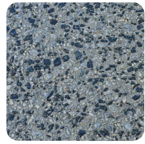
#01 FLOORING EXPOSED AGGREGATE CONCRETE FOR EXTERNAL ENTRY PATHWAYS
