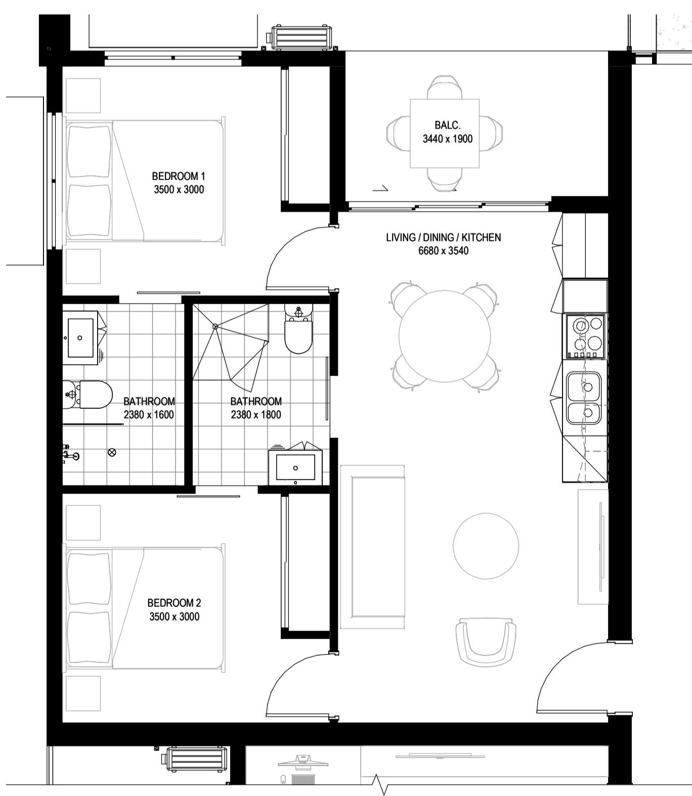
4 2 Bed Serviced Unit - Typical 1 : 50
