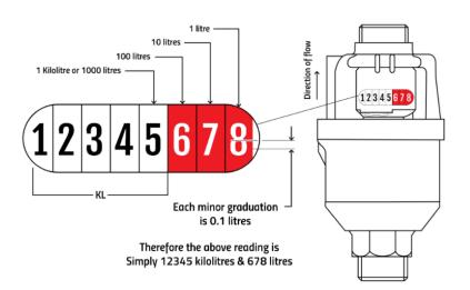
**Smart** meters have numbers to the left and right of a decimal point. The numbers to the left of the decimal point are used for meter reading purposes.
