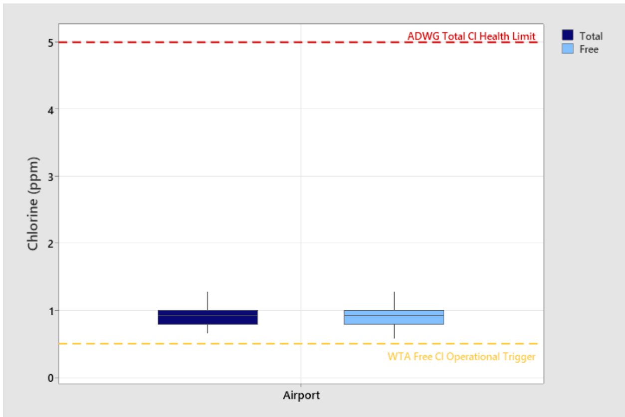
Figure B1(c) Free and total chlorine operational monitoring – Airport Water Supply Scheme
